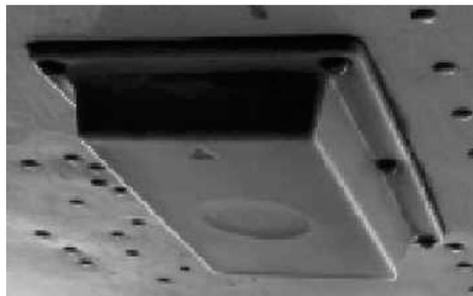
Fig.59- Antena ADF de Loop
