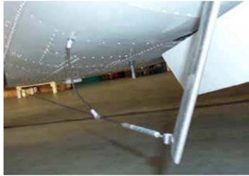
Fig.60- Antena ADF de 'Sense'
