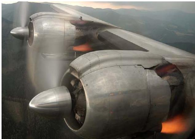
Figura 21 – Motor *turbo-compound* do Lockheed *Super Constellation*
