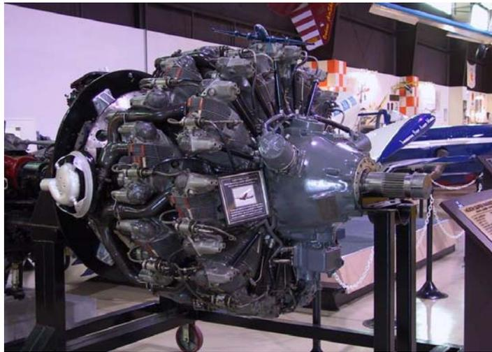
**Figura 3 – Motor Wright R-3350-DA3 turbo-compound de 18 cilindros**
